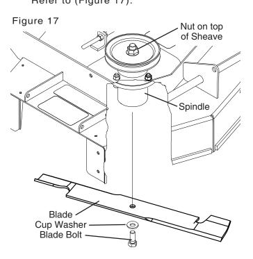
Always use original Bush Hog Parts and refer to the mowers operators manual for blade maintenance.
